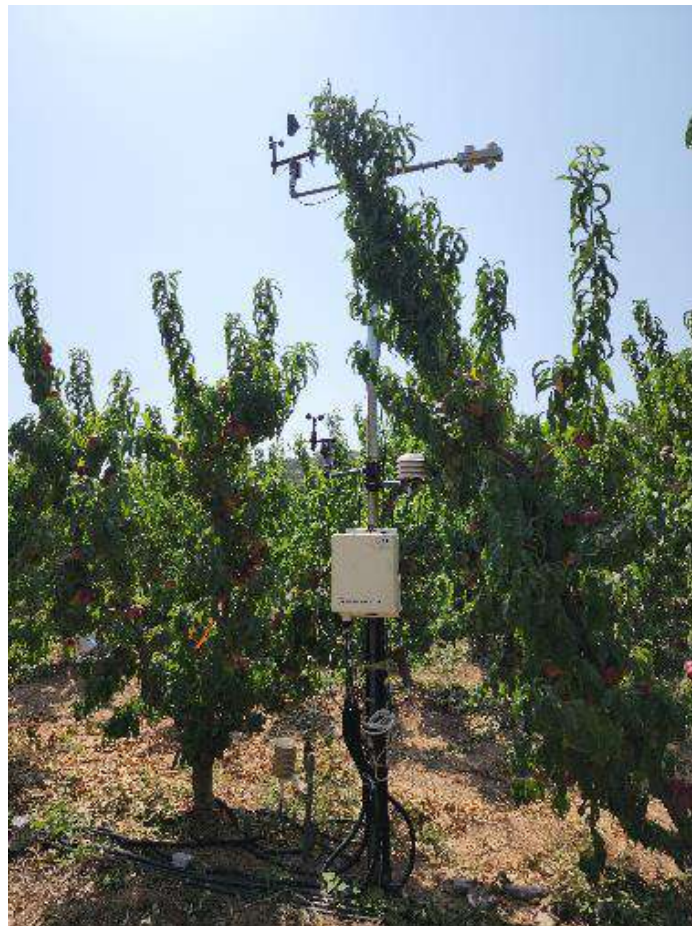
Metrological station (in sun)
